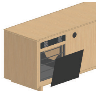
View of back of specialty credenza with access panel, AV rack and thermostatically controlled exhaust fan.
