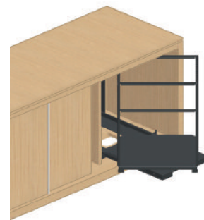
View of front of specialty credenza showing the pull-out and rotating AV component rack.
